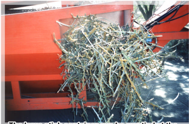
The large stick container can be emptied at the end of each row for easy disposal when the brush is removed at pruning time.
