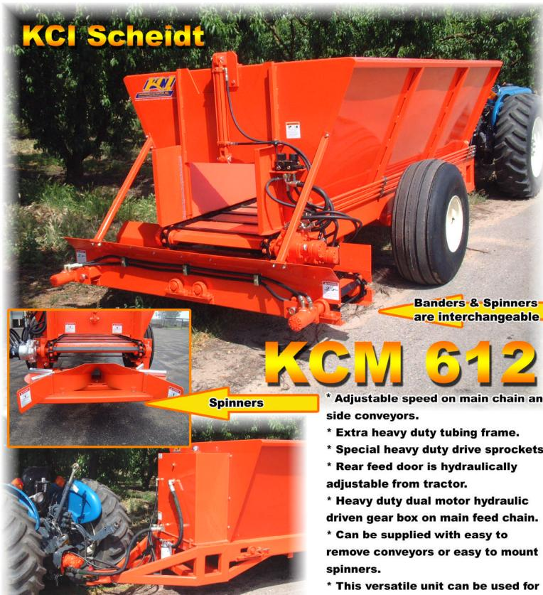
\*Compact self contained hydraulic system with large 80 gallon tank facilitate easy hook and unhook to tractor.
